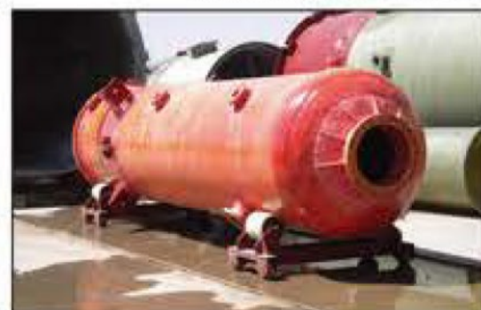
酚醛罐 Phenolic tank
