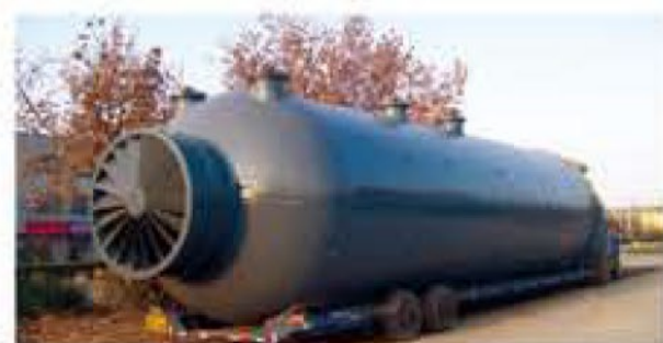
SF干燥塔 SF dry tower
